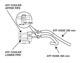
60. Route the hoses installed on the ATF cooler through the hole cut in the left air guide, and fit the ATF cooler into place on the bulkhead. Install the three washerbolts from the kit through the ATF cooler into the threaded holes in the front bulkhead. Tighten the bolts securely.
