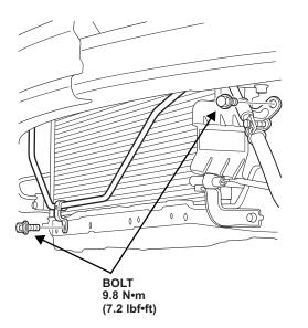
56. Detach the clips, then remove the left air guide.
