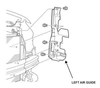
57. Cut the left air guide along the lines as shown. Then remove and discard the cut piece.
