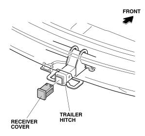
Install the ball mount to the trailer hitch using a hitch pin clip and hitch pin.
