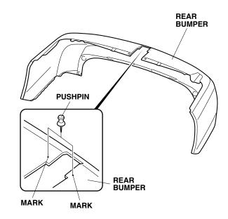
39. While wearing eye protection, drill the rear bumper. First drill with a 3 mm drill bit, and finish with a 10 mm drill bit. Remove any burrs.
