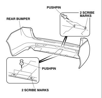
32. While wearing eye protection, drill the front two pierced marks in the rear bumper. First drill with a 3 mm drill bit, and finish with a 10 mm drill bit. Remove any burrs.
