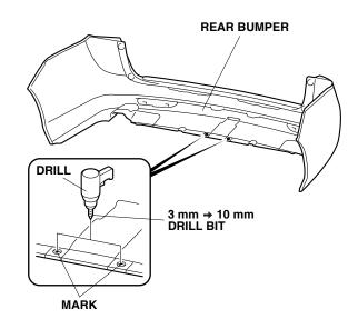
33. Drill the rear two pierced marks in the rear bumper. First drill with a 3 mm drill bit, and finish with a 10 mm drill bit.
