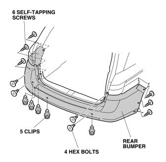
• Release nine retaining tabs on each side.
