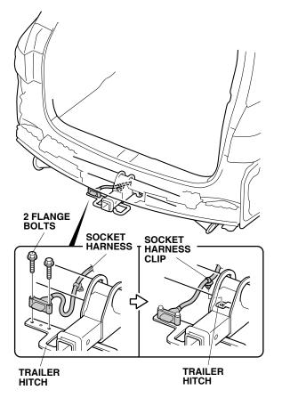
43. Secure the socket harness to the trailer hitch with the socket harness clip.
