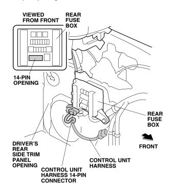
20. Plug the control unit harness 14-pin connector to the
